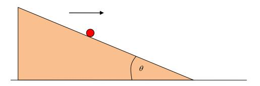
A ball on the wedge remains at rest **relative to the wedge**. The wedge is frictionless.
